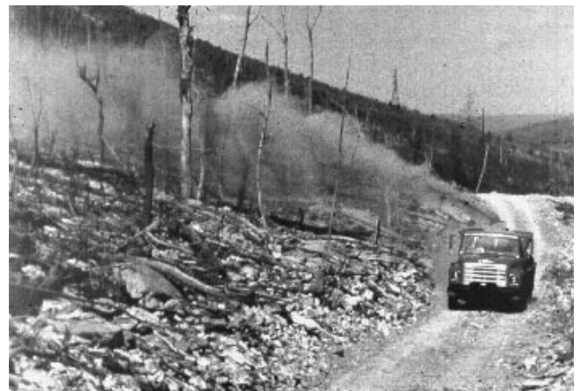
A truck designed to blow flyash and sludge up to 100 feet up the slope.
