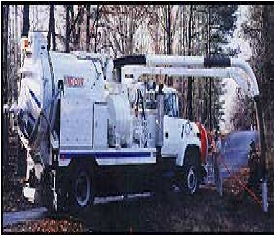
Figure 4.3.7: Jet Vac Truck Cleaning a Sewer
